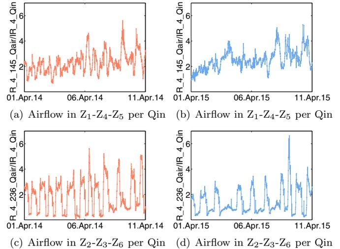
Fig. 5. Line R\_4 - Process operation comparison without (left column) and with (right column) the OPCM, in terms of the cumulative airflow per influent flow-rate in the zones Z<sub>1</sub>, Z<sub>4</sub>, Z<sub>5</sub>, (a) and (b), and in the zones Z<sub>2</sub>-Z<sub>3</sub>-Z<sub>6</sub>, (c) and (d).
