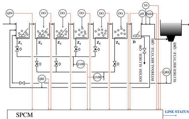
Fig. 2. Activated sludge process at the Mussalo WWTP: Input (in red) and outputs (in blue) for SPCM.
