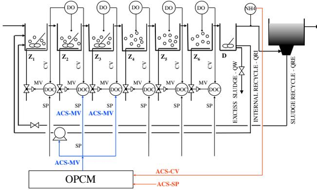
Fig. 1. Activated sludge process at the Mussalo WWTP: Inputs (in red) and outputs (in blue) for OPCM.
