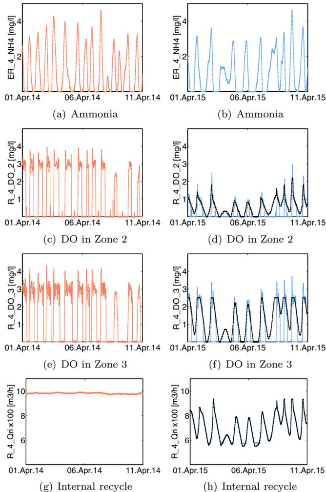
Fig. 4. Line R\_4 - Process operation comparison without (left column) and with (right column) the OPCM, in terms of effluent ammonia from the bioreactor, (a) and (b), dissolved oxygen in zone Z<sub>2</sub> (c) and (d), in zone Z<sub>3</sub>, (e) and (f) and internal recycle, (g) and (h). The black line is the control action given by OPCM.
