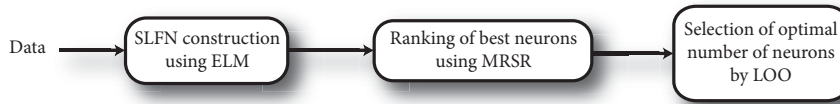
Figure 16: The three steps of the OP-ELM methodology: construction of the SLFN using ELM; ranking of best neurons using MRSR; use of LOO criterion to decide how many neurons are kept.
