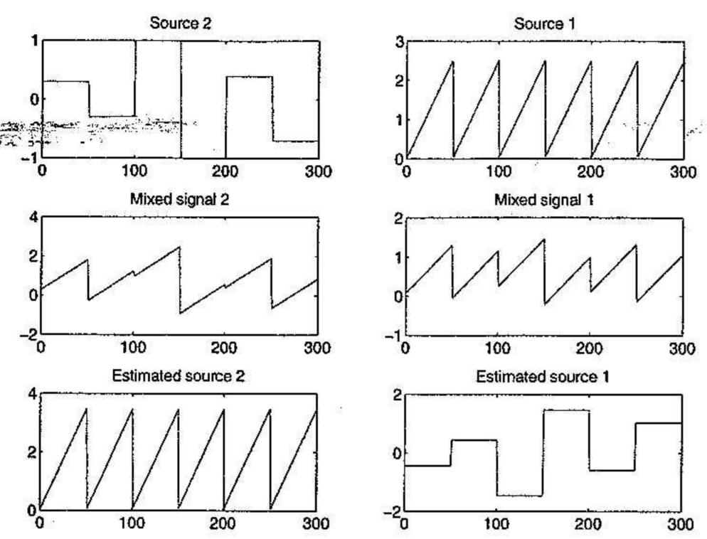
Fig. 1. The results for ICA obtained by optimization in (9) on the Toy example. First row shows the original components, second row, shows the whited mixtures, and the third row shows the estimated independent components.
