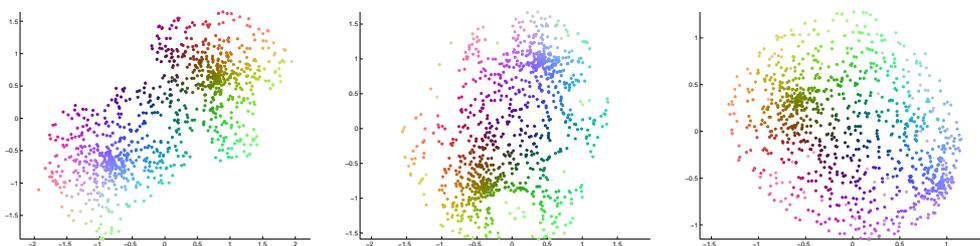
Figure 6: Three projections of a three-dimensional spherical cell with local MDS. On the left, trustworthiness of the projection is maximized by selecting  $\lambda = 0$ . In the middle and right, discontinuity of the projection is penalized as well, by setting  $\lambda = 0.1$  and  $\lambda = 0.9$ , respectively.
